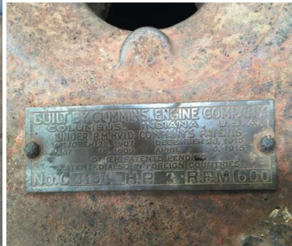
Data plate showing the engine, No.315, was built by Cummins in Columbus, Indiana, with a rating of 3 hp at 600 rpm.
