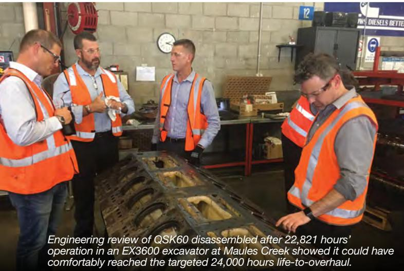
Engineering review of QSK60 disassembled after 22,821 hours' operation in an EX3600 excavator at Maules Creek showed it could have comfortably reached the targeted 24,000 hours life-to-overhaul.
