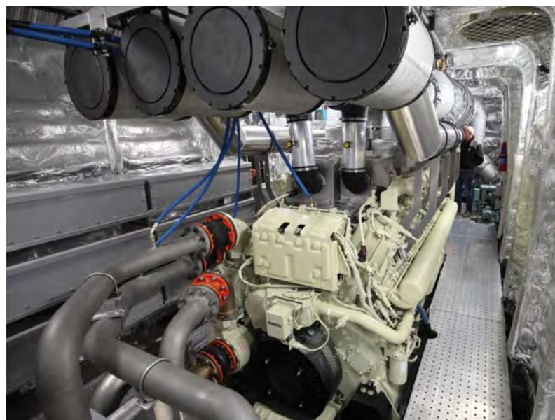
3,600 hp QSK95 fitment in Kilimanjaro VII exceeds Cummins’ installation requirements, reflecting high build quality.
