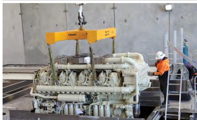
*QSK95 being lowered into the hull last year.*
