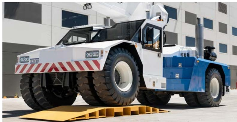
*Humma's dynamic hydraulic suspension automatically levels the crane during lifting.*
