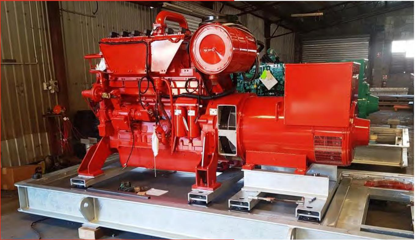
At the start of January 2020, Synchrotech Controls' technicians successfully completed commissioning of the four Type B compliant gensets, each utilising a Cummins KTA19GC industrial gas engine, producing 1.3 MW generator power all up and operating 24/7. The project is also supported by one QSX15 diesel black start unit.
