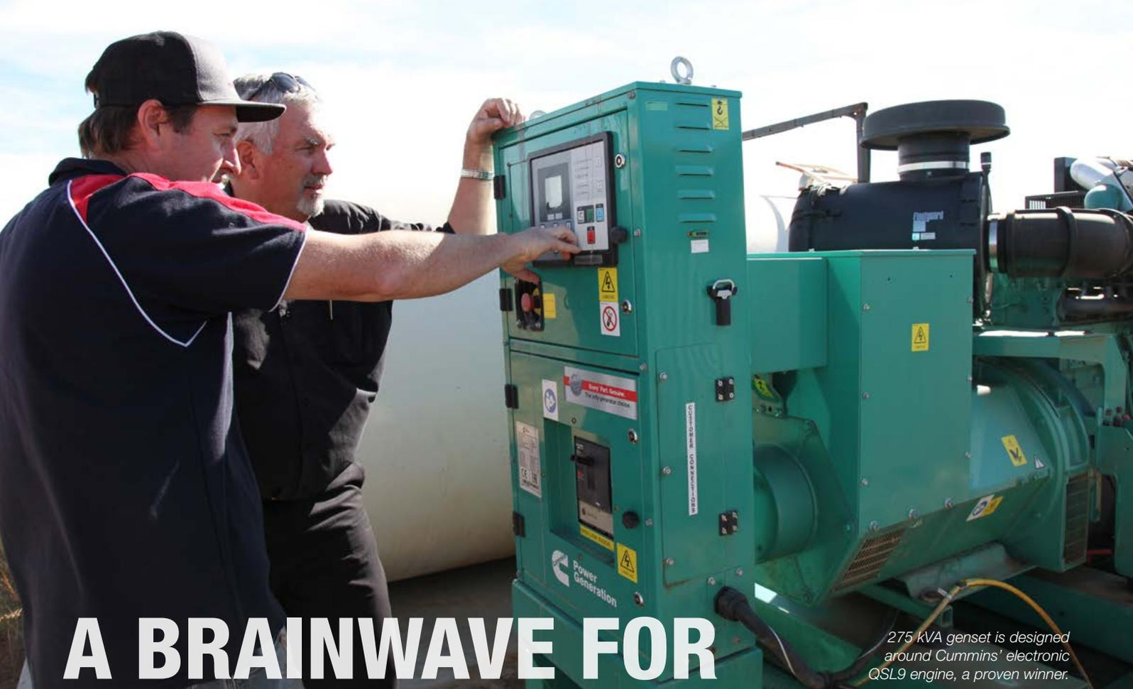
*275 kVA genset is designed around Cummins' electronic QSL9 engine, a proven winner.*
