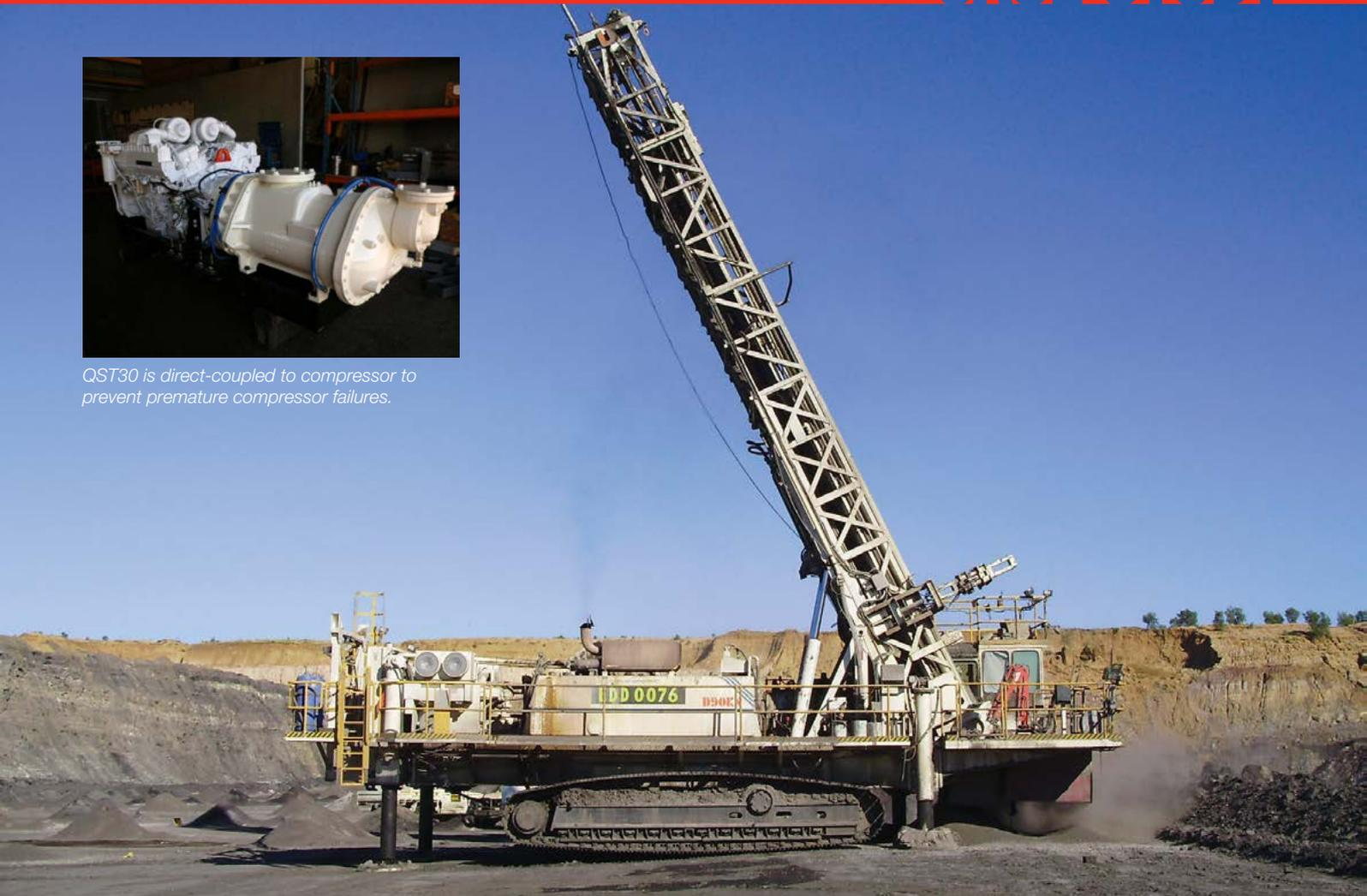
*One of the more than 20 drills have been repowered by Sharps with the QST30.*
