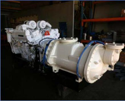
*QST30 is direct-coupled to compressor to prevent premature compressor failures.*
